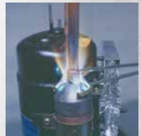
Accumulators can be brazed extremely fast by simply laying the patented "C" style tip near the joint.
